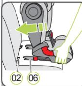
8. Place the child safety seat in driving direction on a vehicle seat approved for use. Ensure that the backrest (14) is flush with the backrest of the vehicle seat.
