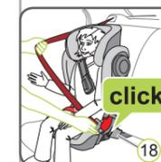
2. Pull out the vehicle belt and guide it in front of your child to the vehicle seat buckle (18).
