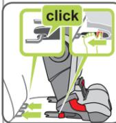
10. Push both ISOFIT locking arms (06) into the insert guides (02) until the ISOFIT locking arms (06) engage on both sides with a clicking sound.
