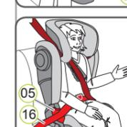
4. Place the diagonal seat belt section (17) and lap belt section (16) on the side of the vehicle seatbelt buckle (18) into the light red belt guide (05) of the seat cushion.
