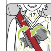
8. Ensure that the diagonal belt (17) runs over the collarbone of your child and is not on the neck and that the key on the belt holder is (03) fully closed.
