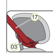
7. Guide the diagonal seat belt section (17) into the dark red belt holder (03) of the headrest (22) until it lies completely in the belt holder (03) and is not twisted.
