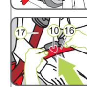
5. Also place the lap belt section (16) on the other side of the seat cushion in the light red belt guide (05).
