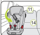
6. Place the XP-PAD (11) in the side of the child safety seat closer to the vehicle door.
